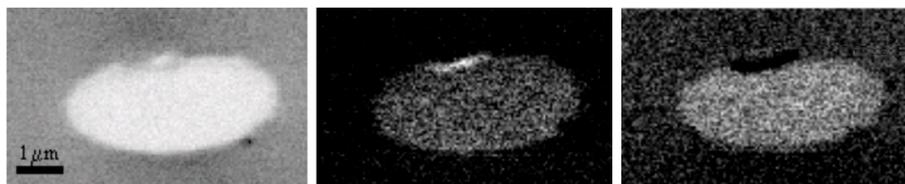
**Fig. 2** (left) Optical density image at 285.1 eV. Component maps of polyester A (centre) and B (right)
