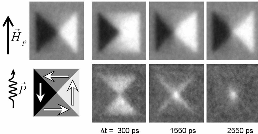
*Dichroic images (upper half) of a permalloy square ( $6 \times 6 \mu\text{m}^2$ ) following the excitation by a field pulse  $H_p$ . Sketch and difference images (lower half) highlighting the changes.*
