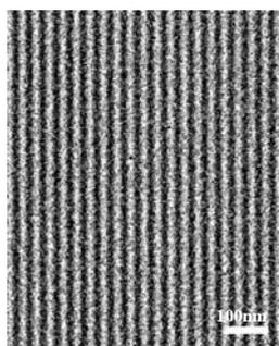
Figure 1. A soft x-ray image of 15 nm test pattern obtained with a 15 nm zone plate at 1.52 nm wavelength (815 eV).
