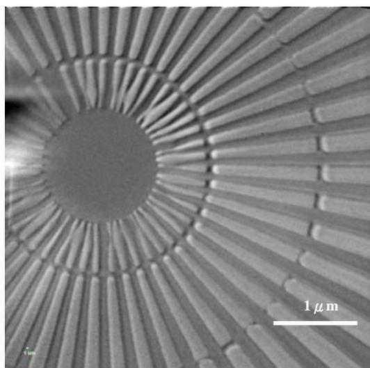
**Figure 1:** The gold spoke-pattern imaged at BL01B at NSRRC by using 3<sup>rd</sup> order diffraction of Fresnel zone plate at X-ray energy 8 keV. The spatial resolution is estimated better than 30nm. Exposure time was 10 minutes.
