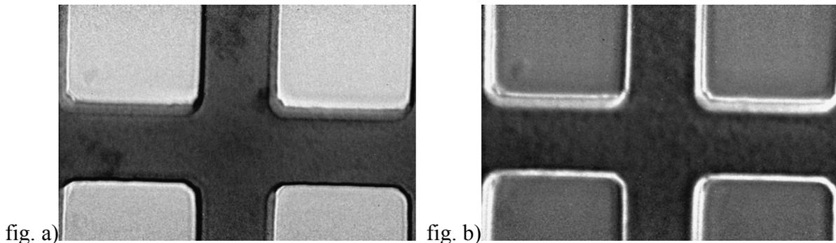
Figures a) and b). Cu #2000 mesh imaged with 1B2 transmission x-ray microscope in bright field and in negative phase contrast, respectively. The width of a bar and a square in the Cu # 2000 is 5 and 7.5 microns, respectively. The field of view is about  $20 \times 13$  micron<sup>2</sup>.
