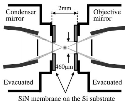
Fig.1 The schematic diagram of a new sample chamber
