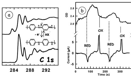
**Fig. 2** (a) C 1s spectra of the oxidized (upper) and reduced (lower) states of polyaniline. (b) (upper) Optical density changes at 283.6 eV (quinoid pi\*) tracked in concert with cyclic voltammetry (CV). (lower) current flows in CV.
