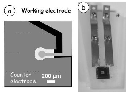
**Fig 1** (a) Details of the 2-electrode cell used for STXM with *in situ* potential control. The chemical state of polyaniline electro-deposited on the working electrode is varied by potentials applied via the spring contacts (b)
