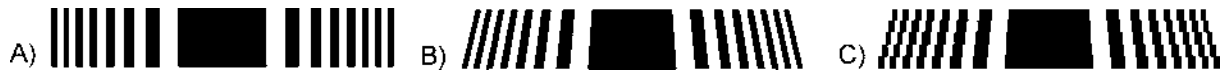
Fig. 1: A) Zone plate with zones parallel to the optical axis, B) Zone plate with tilted zones, C) Zone plate where the local tilt angle of the zones is approximated by 5 layers.
