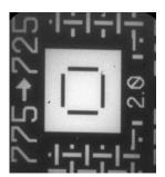
X-ray fluorescence maps of backend copper integrated circuits are presented as an example of non-destructive imaging of sub-surface structures. The x-ray fluorescence camera enables the in-situ location of voids and defects in backend copper ICs without physical deprocessing or ion beam milling preparation and can be performed on whole silicon wafers.
