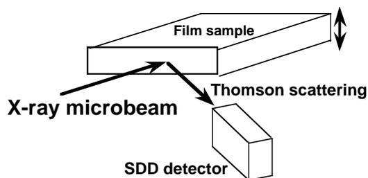
Fig.1 Schematic representation of the X-ray microdiffraction method for film sample.
