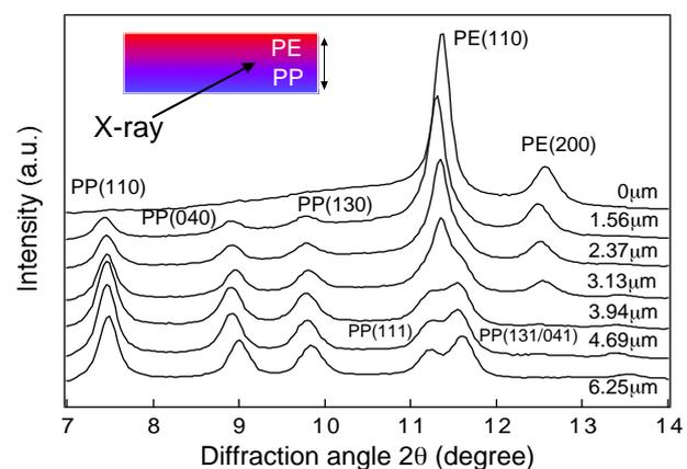
Fig.2 X-ray diffraction profiles of PE/PP laminated film.
