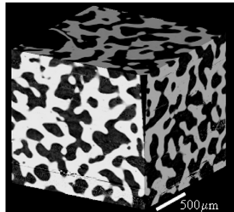
Fig. 1 Three-dimensional image of a PS/PMMA blend obtained by phase tomography.
